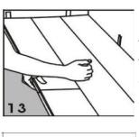
If you wish to remove the flooring, just lift the planks a few centimeters and tap along the joint.
