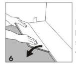
Place the plank at an angle against the plank in the first row, press forward and fold down at the same time. Leave the plank in a somewhat up angled position where the planks start to lock. To make this easier, a wedge with the suitable width can be placed under the plank near the short side.
